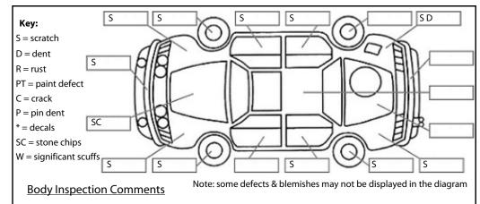
Both front wing mirrors scratched Small holes in drivers seat
