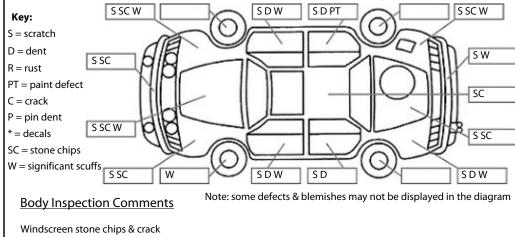
Windscreen stone chips & crack Steering wheel deteriorating Gear selector missing side plastic
