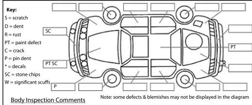
Clear coat peel in patches Pin dent left a pillar
