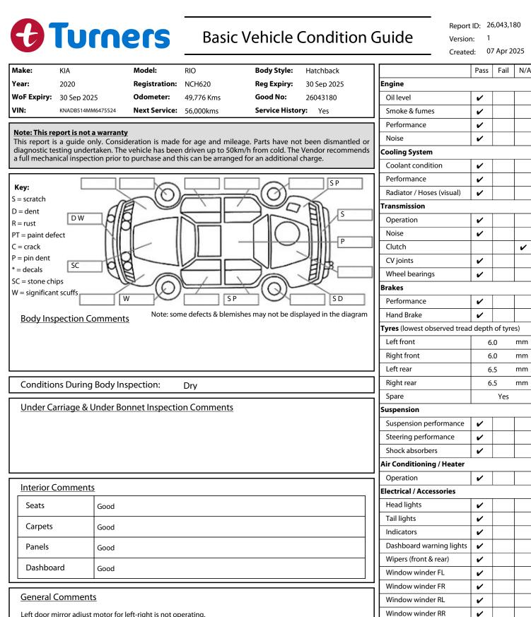
Left door mirror adjust motor for left-right is not operating.
