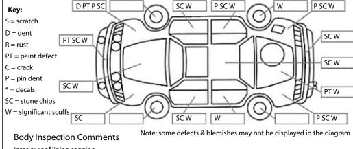
Interior roof lining sagging Bonnet gas struts not holding securely Small chips front screen Scuffing front bumper lip Paint fade/peel vehicle exterior
