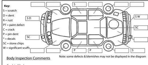
Crack in Windscreen. Rear Air Vent damaged Remote Key damaged
