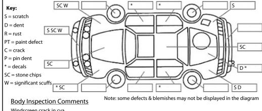
Windscreen crack in cva Lower Ball Joints has play drivebelt tensioner is noisey Both c pillars dented
