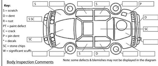
FL fog lamp dummy missing Aftermarket parts fitted on the roof FL park light not working Rear bumper damage, trim insecure Holes on console panel left side
