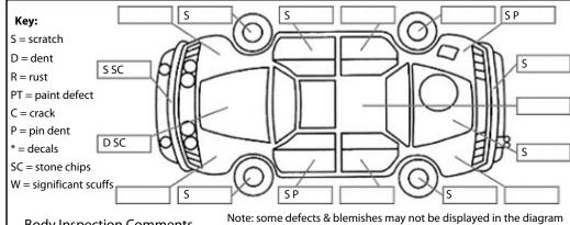
2 x small stone cracks in right side of windscreen. Stone chips in windscreen. Deep scratches on left side sill.
