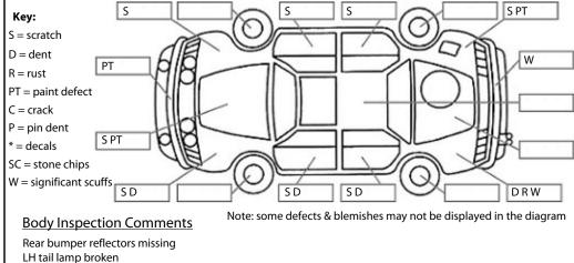
Rear bumper reflectors missing LH tail lamp broken Front bumper trim insecure Rear bumper misaligned
