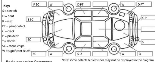
**Body Inspection Comments** Vehicle has puncture repair kit
