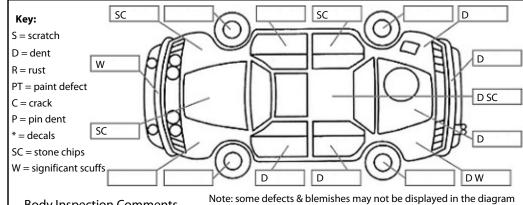
Stone chips front screen. Scuff left rear cab corner and small dent right side. Right inner sill needs painting.
